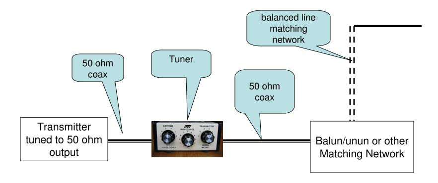
• Depending on the antenna, the tuner may be only for touch-up (okay for internal tuner) or may have to do some serious, wide-ranging matching
