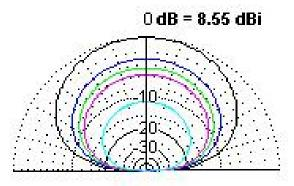
As the dipole is brought lower than  $\frac{1}{2} \lambda$  above ground, the take-off angle increases until the antenna becomes NVIS
